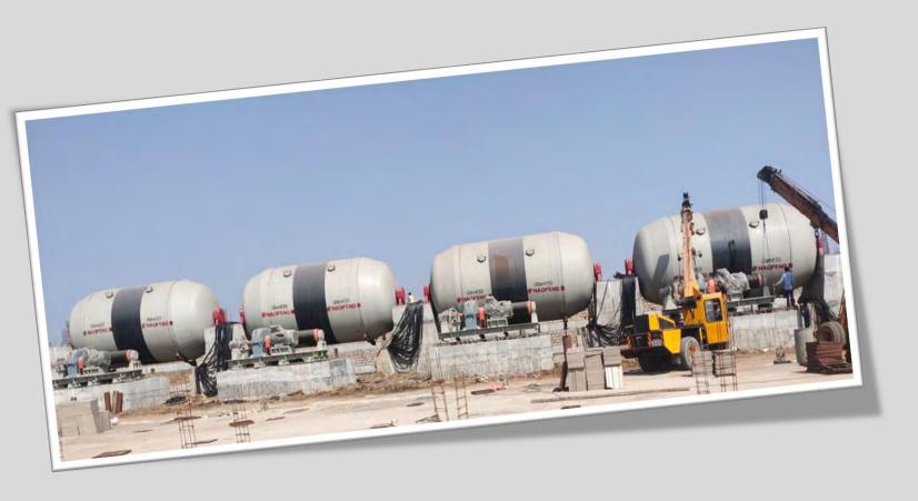
9 Ball mills each of 60 ton capacity, equipped with lining from **SACMI ITALY** Installed for 1<sup>st</sup> Time in Asia from **HAOFENG**, which is well known for its energy efficient Ball mills. Output of which gives you accurate & proper grinding material. Out of 9 ball mills few will be assigned for few specific colors like black ,white & multicolor.
